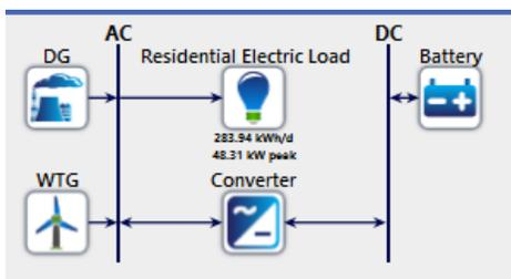
Fig. 1. The wind-diesel micro-grid system architecture
