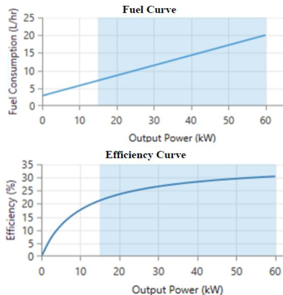
Fig. 3. Fuel and efficiency curves of selected diesel generator
