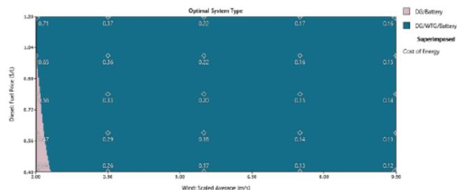
Fig. 6. Optimum cost of micro-grid at interest rate of 3.3% and maximum capacity shortage of 0.0% at different sites across Nigeria.
