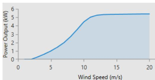
Fig. 2. Power characteristics of Hummer H6.4-5kW wind turbine generator
