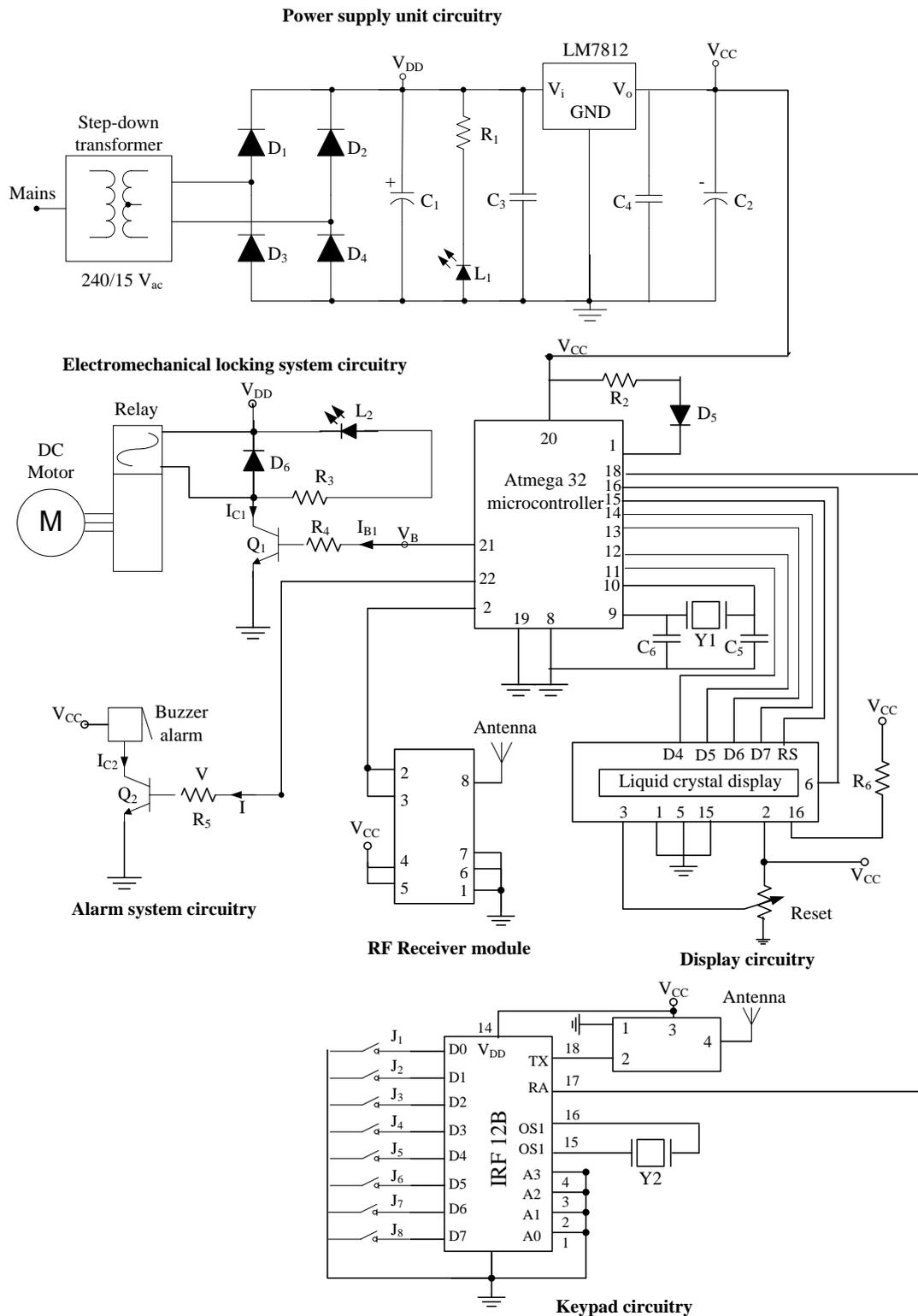
Fig. 2: Schematic of the RFID-based security design setup
