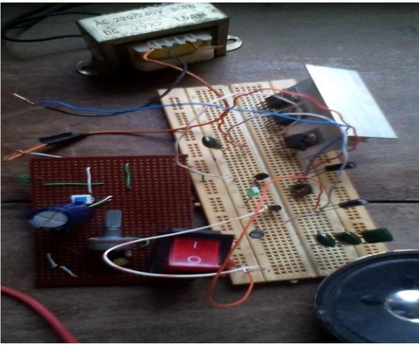
Fig. 4: Bread boarding of the designed circuit
