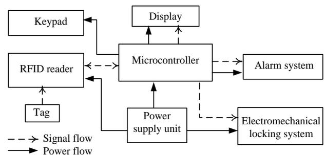
Fig. 1: Architecture of the proposed RFID-based security system
