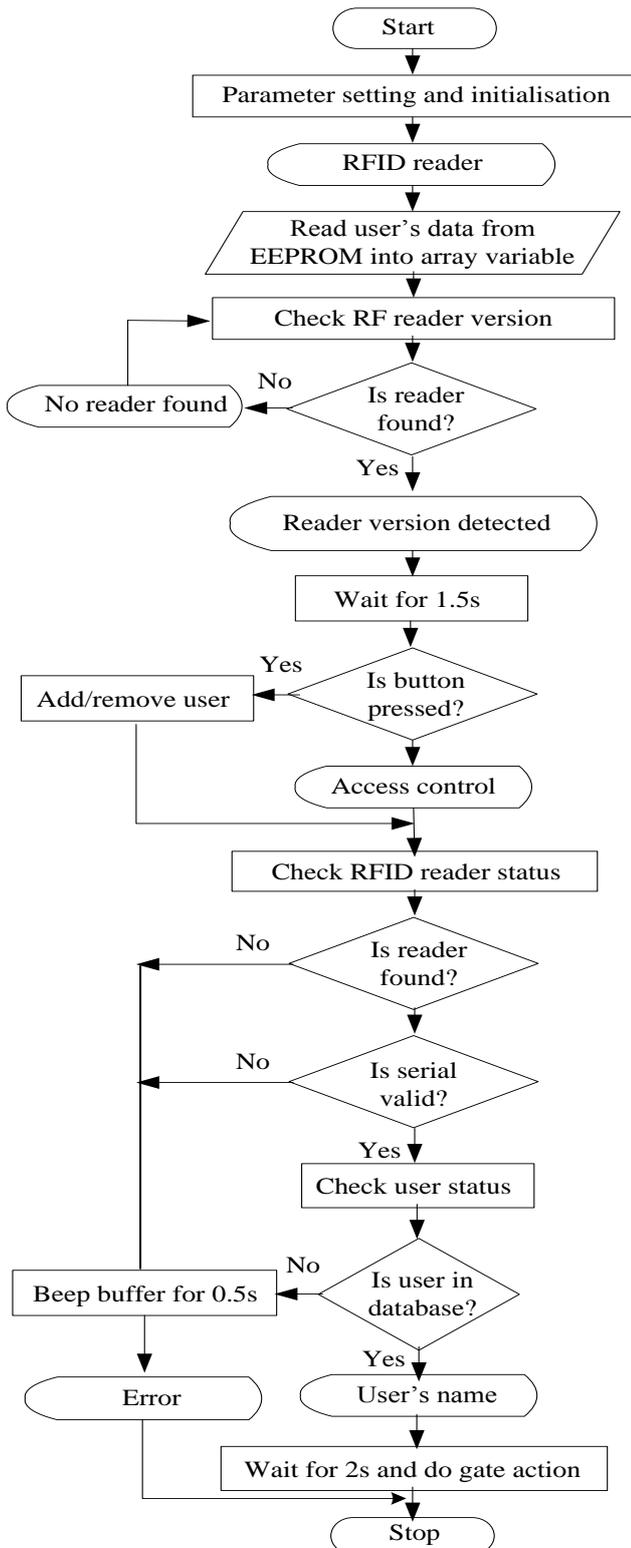
Fig. 3: Control system is the RFID-based security system
