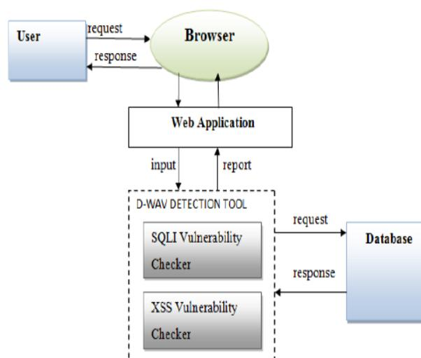
Figure 4. D-WAV system architecture (Singh et al., 2015)
