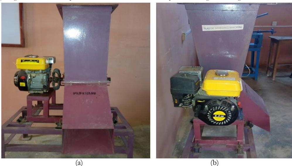
**Figure 4.** Pictorial views of the fabricated plastic film granulating machine (a) front (b) side.
