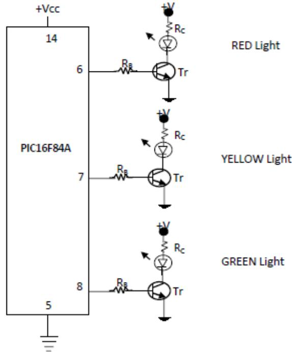
Figure 3: Diagram of Light Indicator
