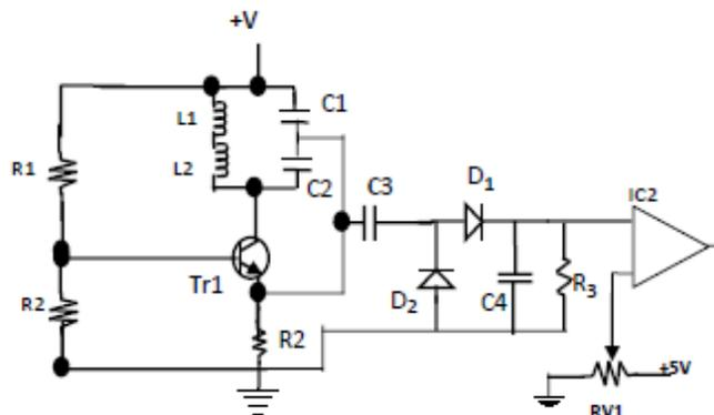
Figure 4: Vehicle detection circuit
