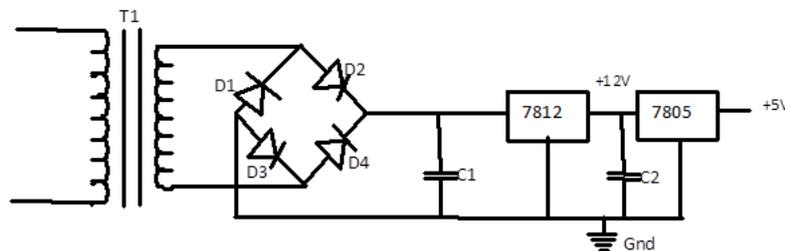
Figure 2: Power supply circuit
