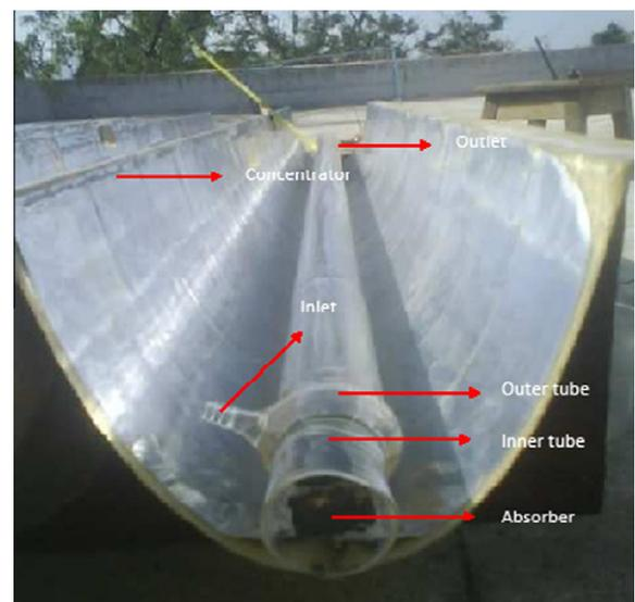
Fig. 4. Pictorial view close-up of tubular solar still.
