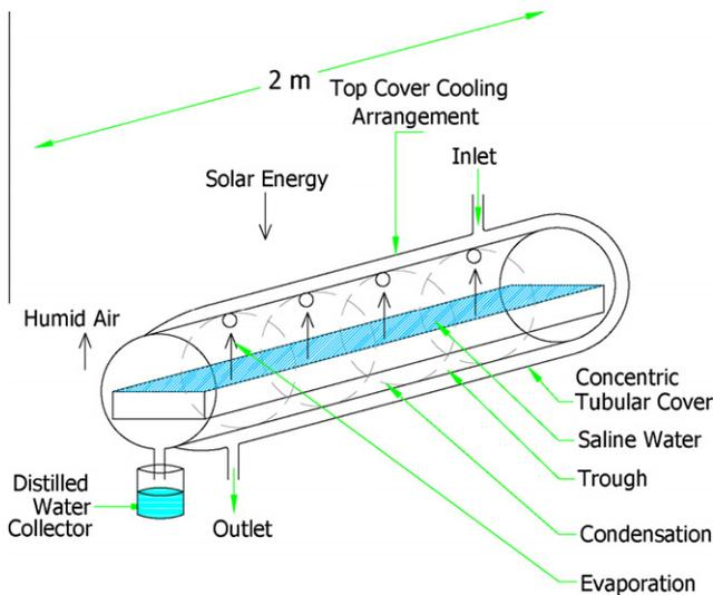
Fig. 3. Schematic view of experimental setup.
