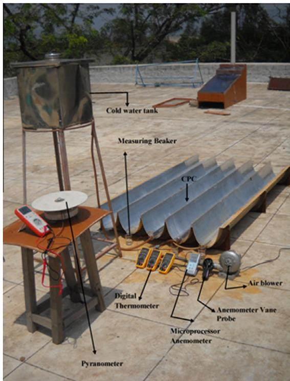
Fig. 5. Pictorial view of compound parabolic concentrator tubular solar still.
