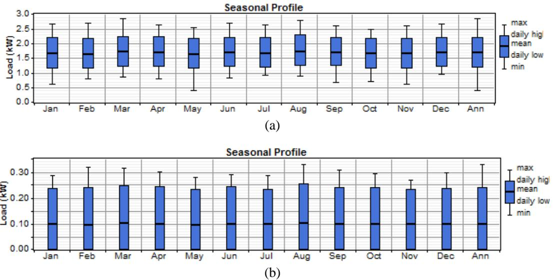
Fig. 2: Seasonal electric load profile of the mobile telecommunication site under study (a) DC (b) AC
