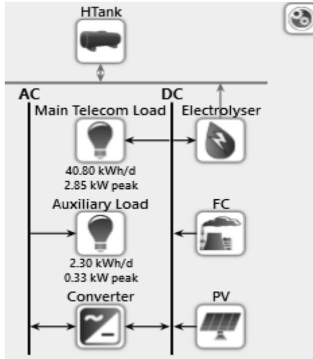
Fig. 3: Process simulation architecture of the PV/FC hybrid system under study
