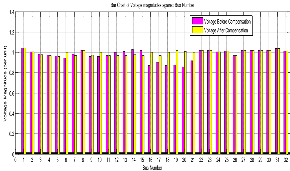
Figure 3: Voltage profile magnitude of the Nigerian 330kV, 32-bus network before and after compensation
